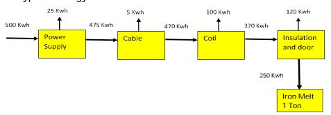
Above diagram shows energy requirements for melting 1 ton typical iron scrap in about 40 to 45 minutes. Tubular copper coil receives heat from two sources:
