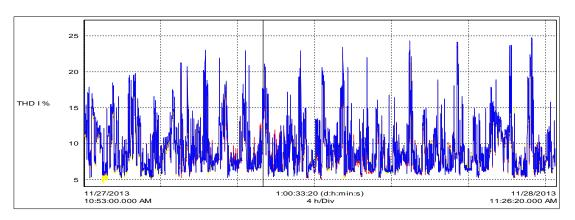
Above recorded data shows that these harmonics are between 12 to 20% and at times they reach even 25%. These readings are obtained on 24 hours basis and as such show all possible load cycles for a typical load pattern.
